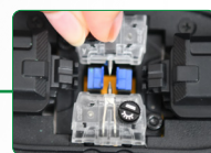
The electrodes can be replaced by screwing it gently without tools
